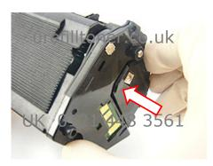
As long as end plate is pushed on firmly there's no need to fix it into position. As soon as it's back in the machine, the plate is held firmly in place. But be aware that the end plate isn't fixed on and that it could be a source of problems if it worked loose.
